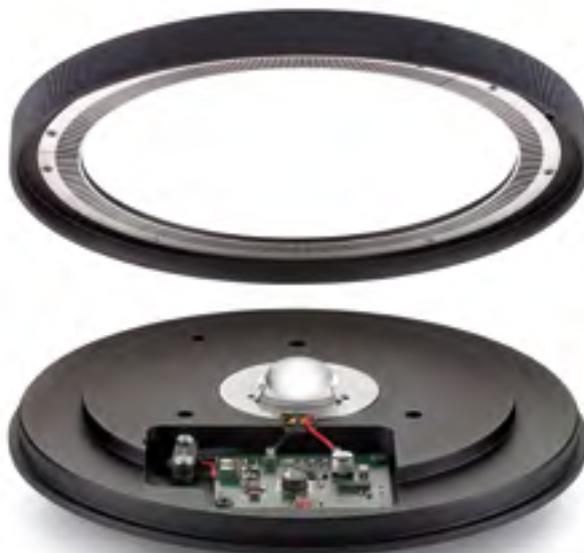
Rotary dimmer mounted on Eva's base with infrared sensor to detect rotation and adjust light intensity.
