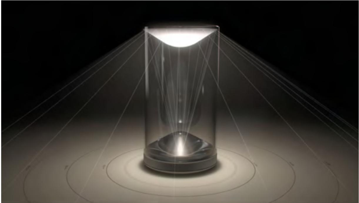
In Eve and Eve, the light flux is projected through a holographic filter, a small primary lens and a large secondary lens on the upper opaline cone, while the LED source remains hidden. Both lamps also have a tactile dimension: while with Eve the light is dimmed by a touch dimmer, with Eva it is dimmed by a rotary dimmer, which, thanks to an encoder system (an infrared sensor to detect rotation), allows the light intensity to be precisely controlled by manually actuating the ring on its base.
