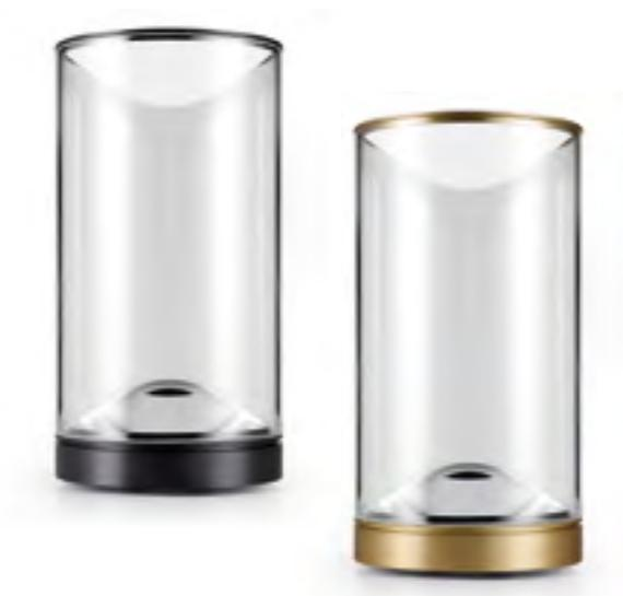
A natural development of Eve, Eve is a floor lamp similar to its big sister, but smaller in size and with a reduced light emission. Eve is a lamp with indirect light: the light source housed in the base emits a beam of light upwards, which passes through a PMMA lens, pointing at the upper conical reflector that acts as a diffuser. Dual-intensity touch dimmer on the base.
