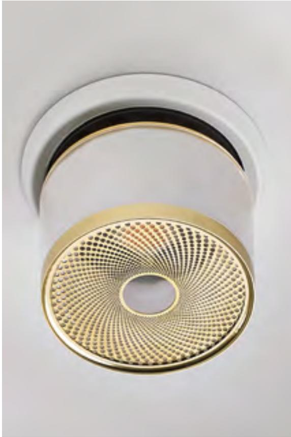
The lower filter made of photo-etched brass foil enables glare reduction and optimal light distribution. The dissipation system, developed and produced inhouse, guarantees the correct operating temperature of the LED. Both the heat sink and the central structure of the lamp are made of turned aluminium using the latest technologies of numerical control (CNC) machines.
